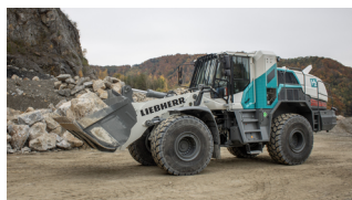
Practical testing of hydrogen-powered wheel loader in Gratkorn © STRABAG / Stefan Bock
